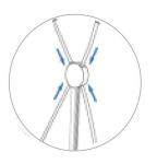
Insert top and bottom graphic arm poles into holes on support pole
