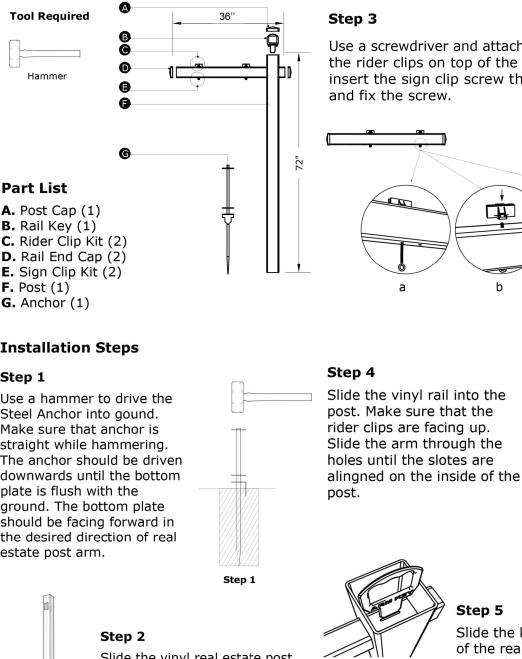
Use a screwdriver and attached screws to fix the rider clips on top of the post arm. Then insert the sign clip screw through the arm, and fix the screw.
