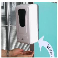
Wave hand under sensor to test dispenser
