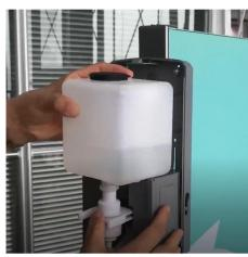
Insert sanitizer tank into the housing
