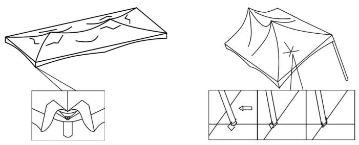
**VII**: Insert all the legs to make the tent stand up,and then fasten the ratchet ropes.
